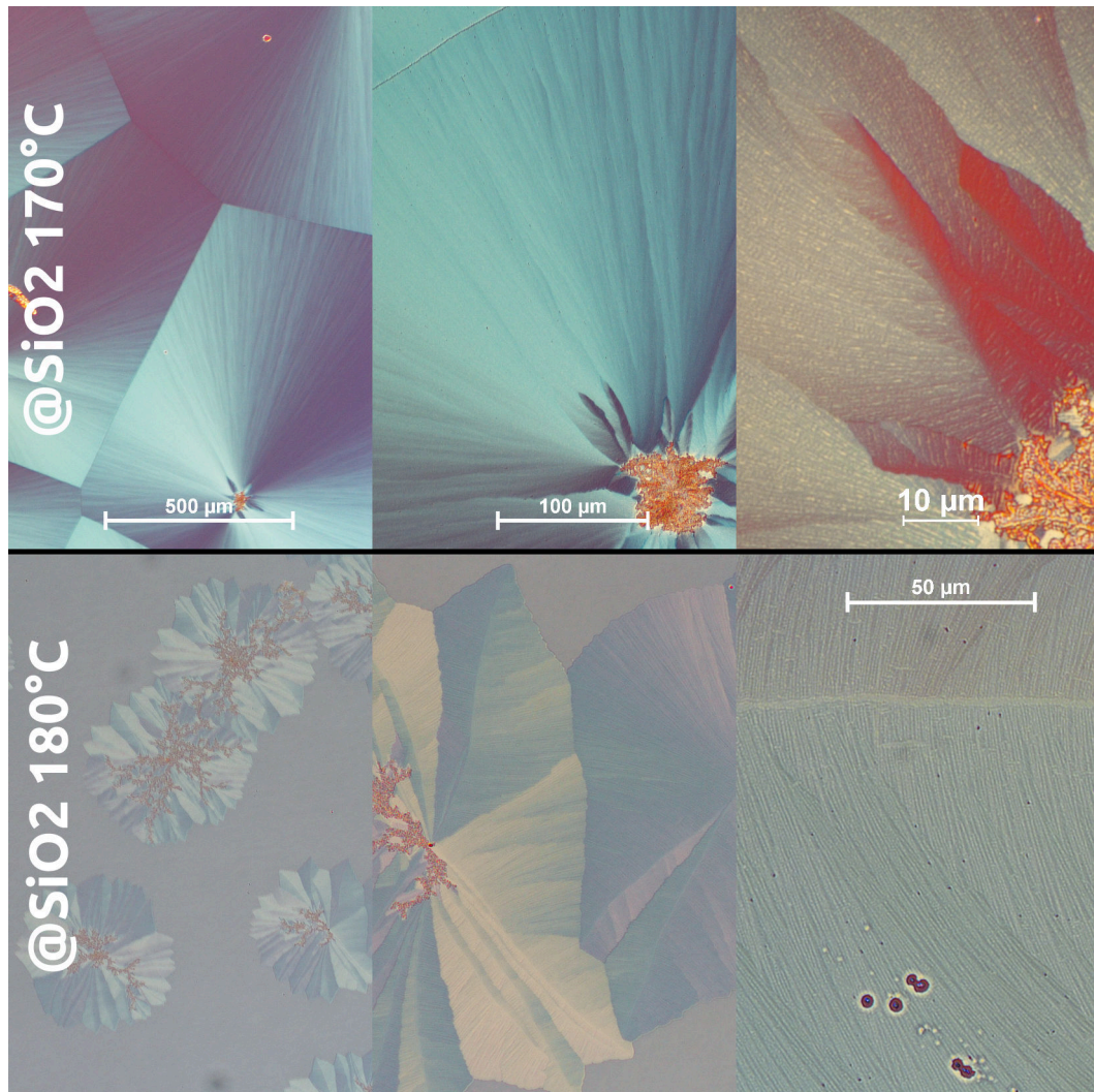
Figure 4.22: Types of rubrene orthorhombic spherulite crystallites (seed thickness: 20 nm): top: Films processed at 170 °C usually grow into solid spherulites with a semi-circular symmetry. bottom: Films processed at more than 180 °C usually grow into ray-like broken spherulites.
