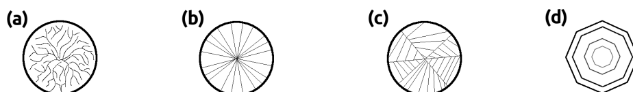
Figure 4.1: Different types of crystallites: (a): dendritic spherulite with strong branching, (b): dendritic spherulite with low branching, (c): crystallite consisting of several sub-grains, (d): platelet type single crystal.
