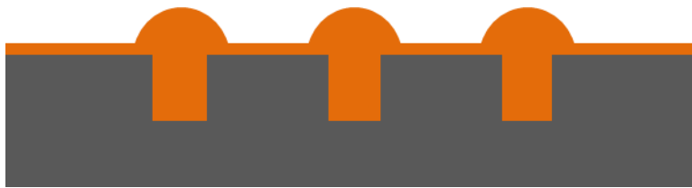
Figure 1.2: Representation of “over-fill bumps” which are bumps that form over features that undergo superfilling (see reference 12). They are caused when the electroplated material continues to deposit at a higher rate than the wafer field after the feature has been filled completely.
