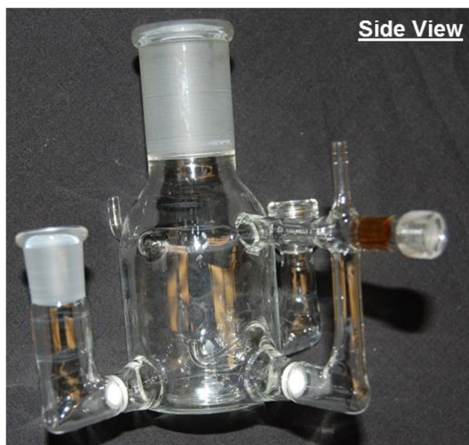
Figure 2.1: One compartment glass Electrochemical cell. A valve is used to direct gas flow for sparging solution or for maintaining atmosphere. The counter electrode is separated via medium glass frit and a Luggin-Haber capillary connects the main cell to the reference electrode.
