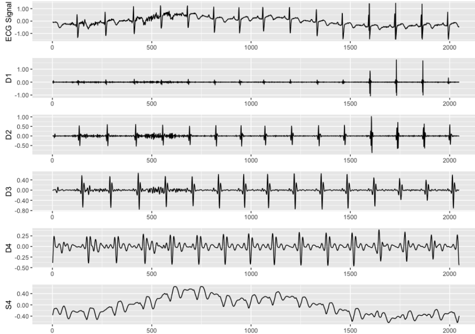
Figure 6: The shift invariant MODWT. Movement of coefficients align across resolution levels using four-level wavelet MRAs, utilizing the “la8” Daubechies wavelet filter, of an ECG signal as presented in Percival and Walden [73].
