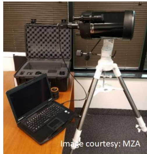
Figure 1. DELTA turbulence profiling system.
