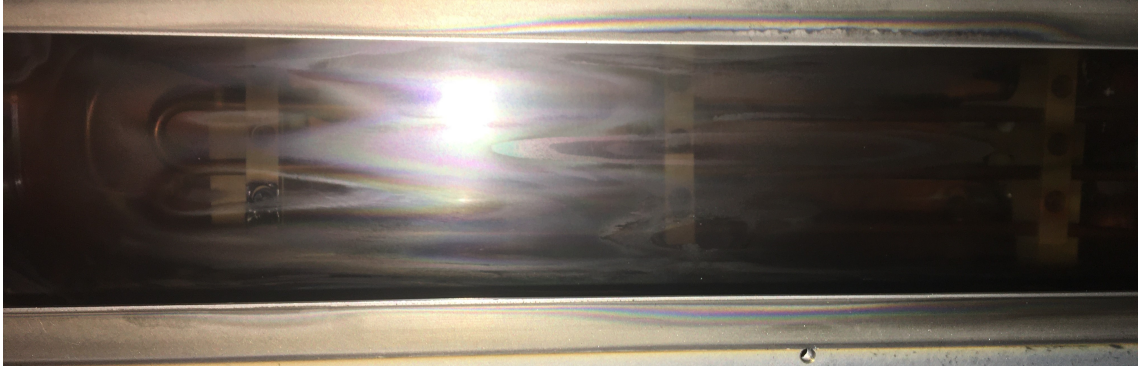
Figure A.1: Image of REVAN’s dielectric window after E-mode degradation. The antenna can be seen on the other side, but is covered by deposition that will reduce the power transferred from the antenna to the ion source.
