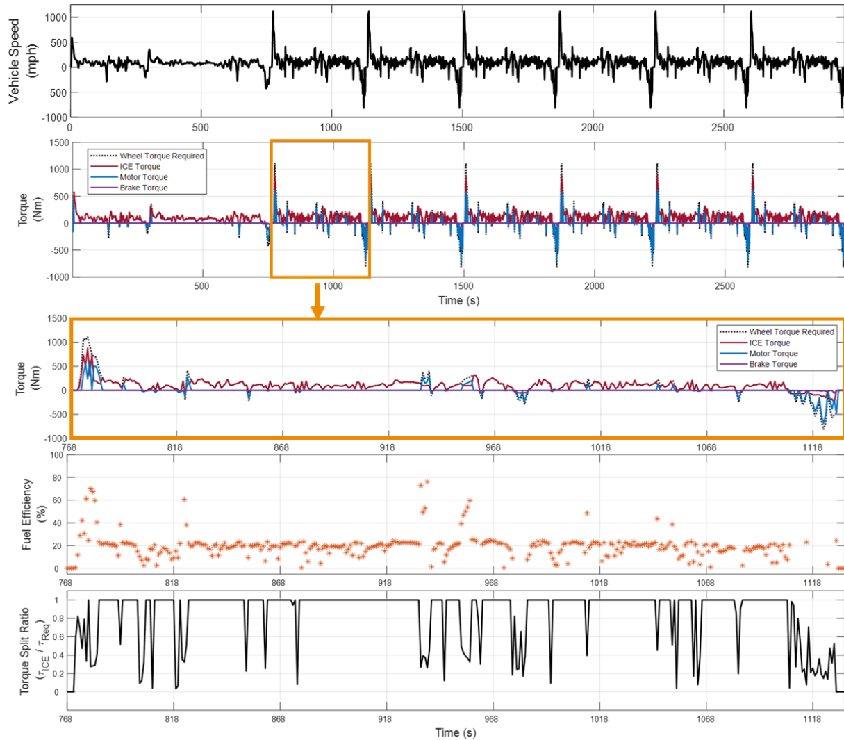
Figure 60: Torque Production of Highway Driving Portion of the EMC Highway Cycle
