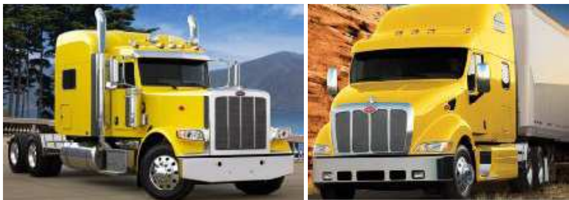
Figure 5.3: The traditional Peterbilt truck (left) and the SmartWay Peterbilt truck (Source: Peterbilt Truck manufacturer's website)
