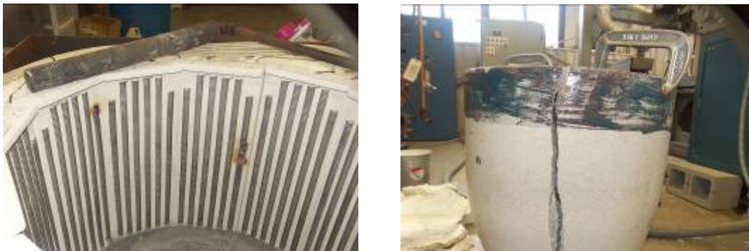
Figure 4-25: Damaged Inductors and Broken Crucible
