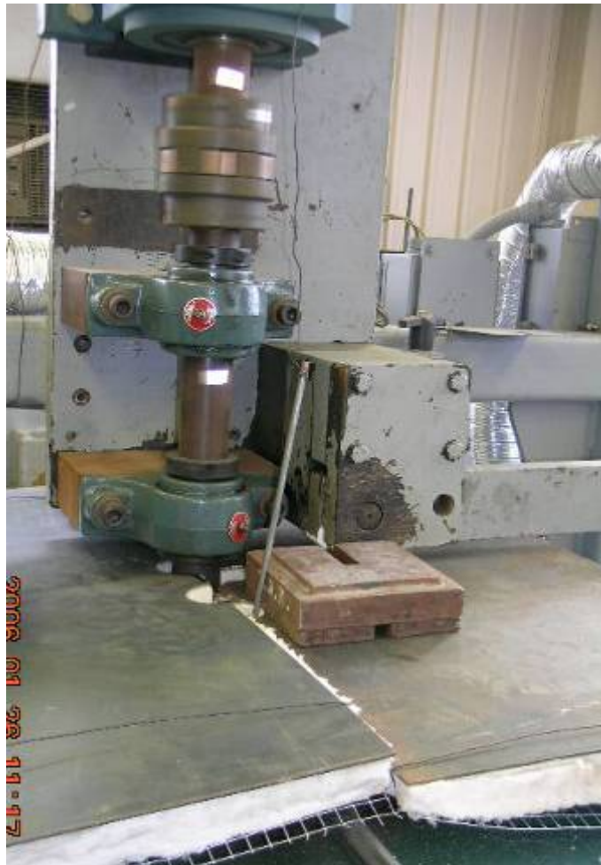
Figure 4-24: Test Rig during 10 hour Stellite 21 Test
