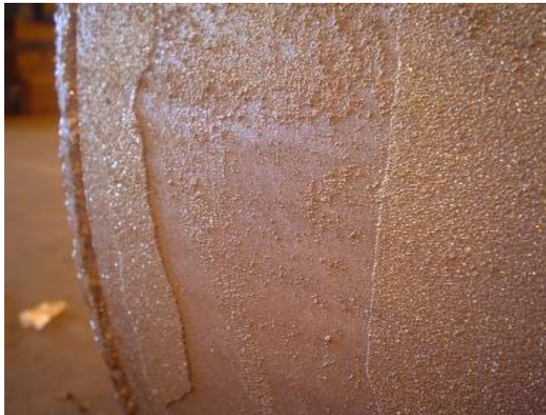
Figure 4-1: Dross build-up on the Sink Roll surface used in the Zn-55%Al CGL.
