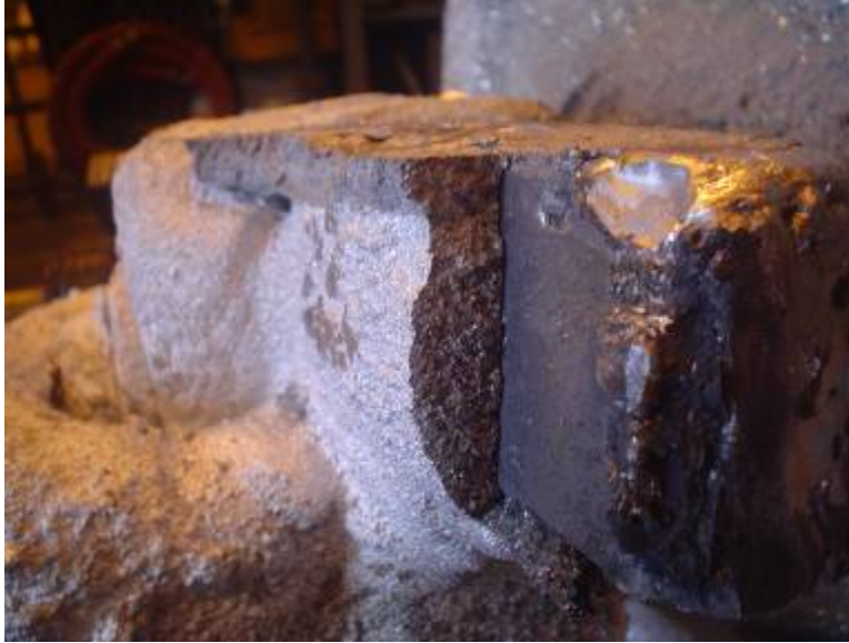
Figure 4-2: Dross build-up on the Sink Roll Pinion arm used in the Zn-55%Al CGL.
