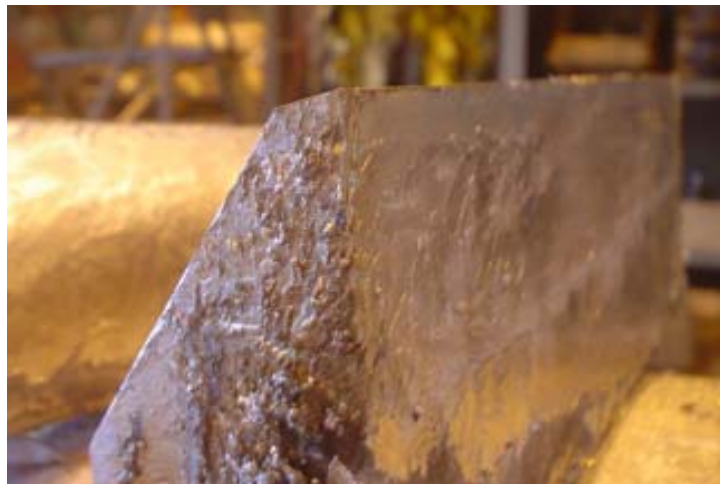
Figure 4-11: Worn out Scraper Blade after ~7 days in GL line.
