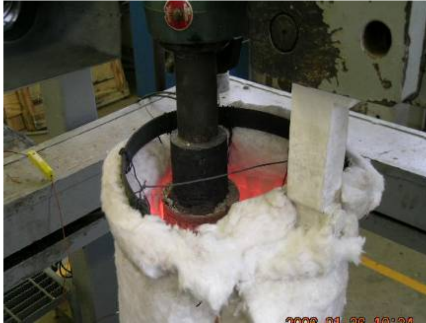
Figure 4-19: Preheating of the Roll and the Scraper Assembly.
