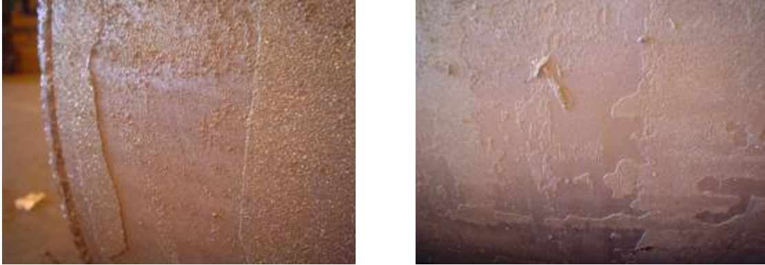
Figure 1-2: Sink Roll Surface Degradation Due to the agglomeration of Dross Particles
