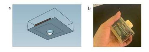
Fig. 3 - (a) Bottom view of the casing design; (b) hardware system of CTAPMS
