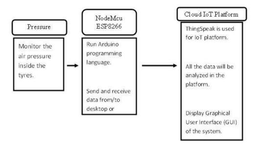
Fig. 2 - CTAPMS block diagram
