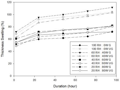
Fig. 1 - Thickness swelling of particleboard
