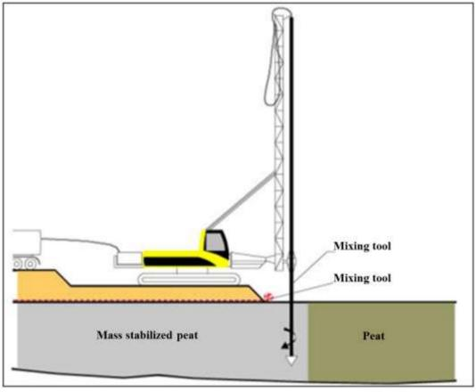
Fig. 2 - Mass stabilization process on peat
