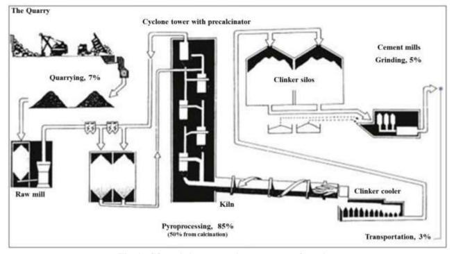
Fig. 1 - CO<sub>2</sub> emission process in cement manufacturing
