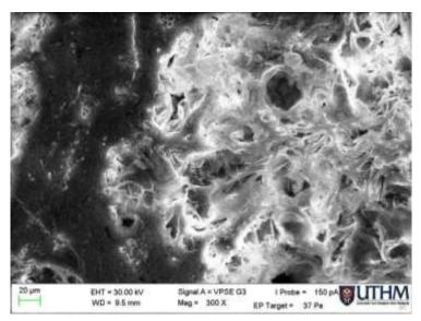
Fig. 6 - Microstructure image for untreated peat soil
