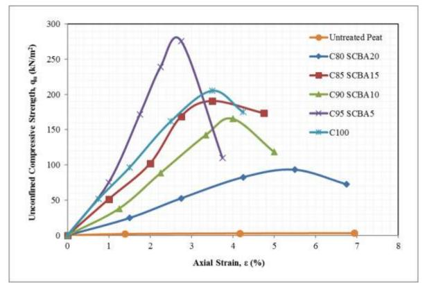
Fig. 5 - UCS Test for 28 days curing
