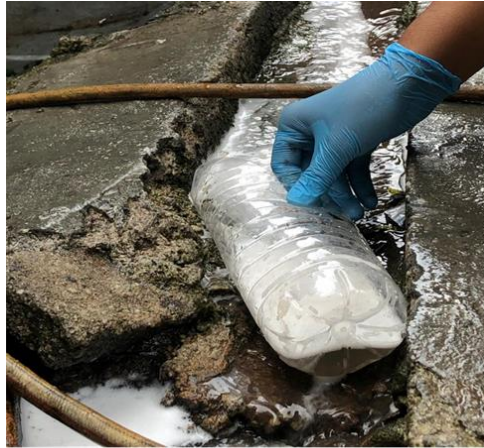
Fig. 2 – Drainage outlet of car wash service, which is the sampling point
