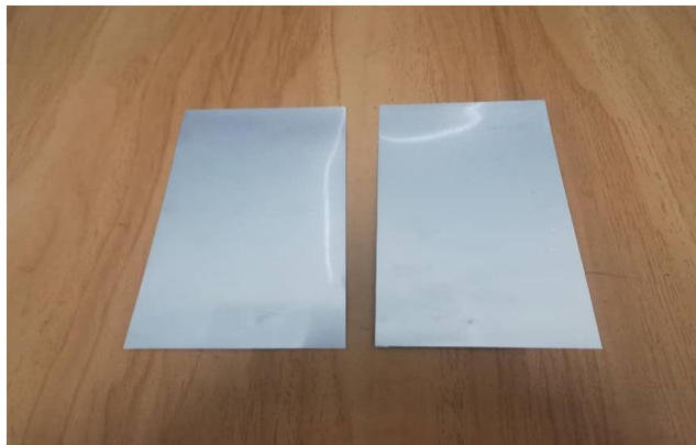
Fig. 3 – Aluminium electrode (left) and stainless steel electrode (right) used for the electrocoagulation process
