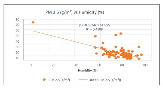
Fig. 4 - Graph of correlation between  $PM_{2.5}$  and humidity (%) for phase 2 at Station B
