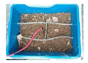
Fig. 7 - Top view of soil area with drip system and moisture sensor
