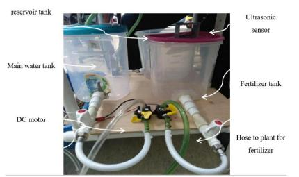
Fig. 6 - The automated solar powered irrigation and fertigation system
