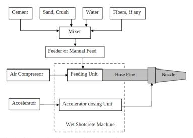
Fig. 1 - Schematic diagram of the wet-mix shotcrete methodology
