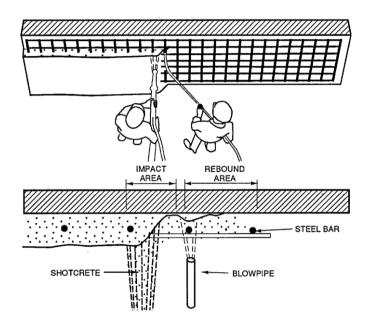
Fig. 2 - Application of shotcrete to the pre-installed wire mesh (After Gideon, 1993)
