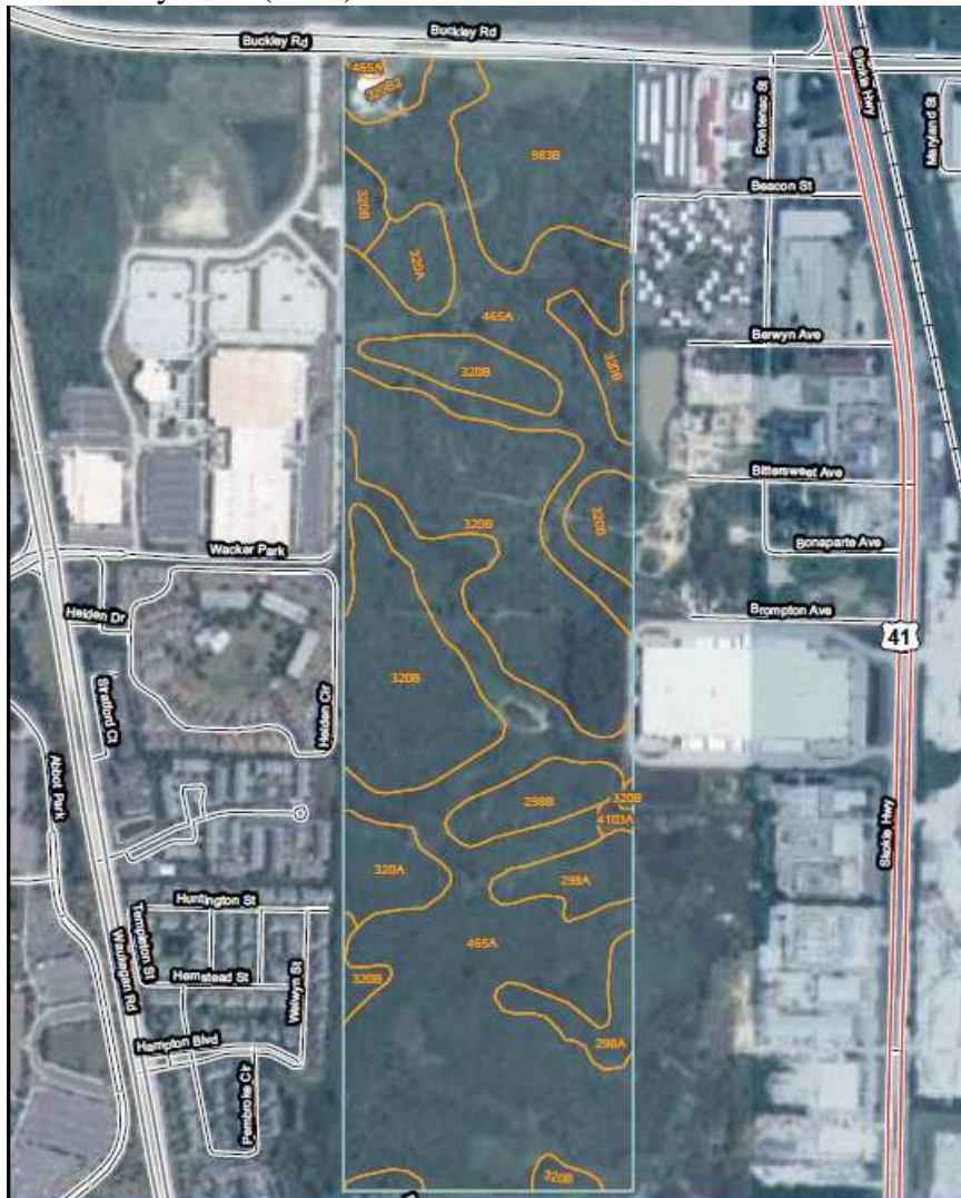
Figure 3. Soils map of the North Chicago Wetland Mitigation Site. The site is outlined by a thin blue line and each soil type is delineated by an orange polygon. The code found in the middle of each polygon corresponds to the soil type found in the legend. All information is adapted from Soil Survey Staff (2010).
