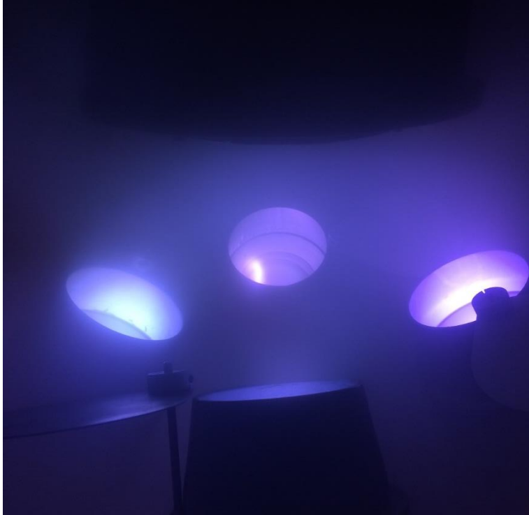
Figure 3.1: photograph of sputter chamber during sputtering of a HEA via four sputter guns (bottom) aimed towards a substrate (top).
