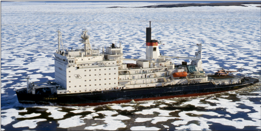
Shallow-draft nuclear icebreaker Taymyr, built in Helsinki and St. Petersburg, in operation since 1989, with its sister ship Vaygach, (not pictured). (GRID-Arendal/Flickr, www.grida.no/resources/3635 )
