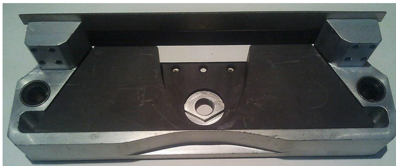
Figure 1: A representation of the bowtie filter module along with its Aluminum holder used in the General Electric LightSpeed™ Volume Computed Tomography scanner.
