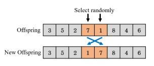
Fig. 10. Illustration of Neighborhood Structures N<sub>4</sub> (Transpose).
