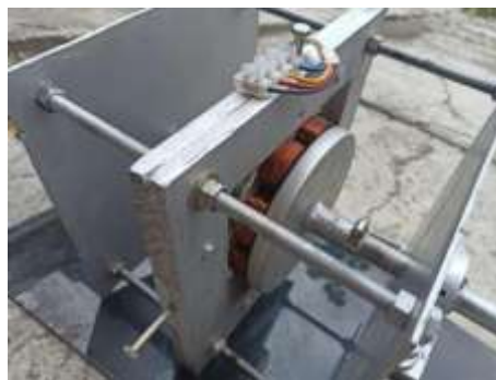
Gambar 11. Generator Tampak Samping
