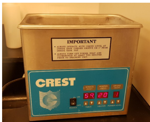
Figure 3.20: Tool for lift-off, which offers sonic energy.
