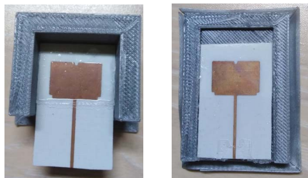
Fig.3. a) Antenna with half PDMS, b) antenna with full PDMS.
