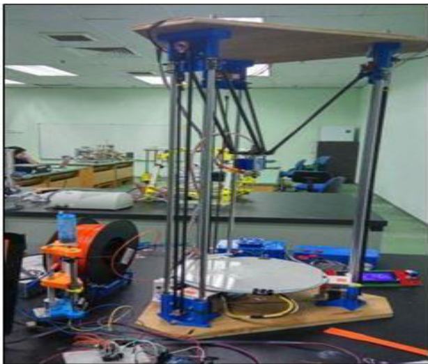
Figure-2. Fused Deposition Modelling (FDM) used to print the product.
