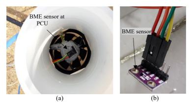
Figure 6. Power converter unit (a) and Bosch BME280 sensor (b).
