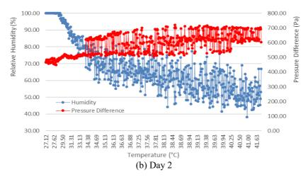
Figure 11. Variation of humidity and pressure difference as function as temperature.
