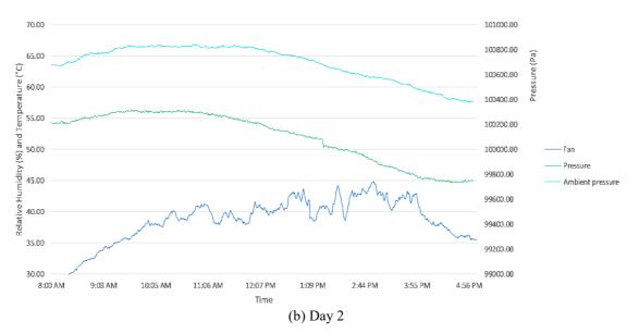
Figure 9. Pressure, relative humidity (RH) distribution at power converter unit (PCU) and along with ambient pressure.
