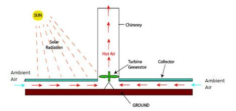
Figure 1. Solar updraft tower concept.
