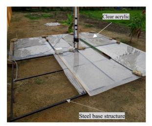
Figure 3. Collector structure using steel with clear acrylic as a collector.
