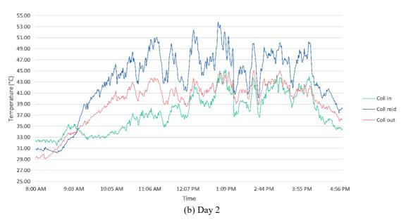
Figure 7. Temperature at a different location under the collector area.
