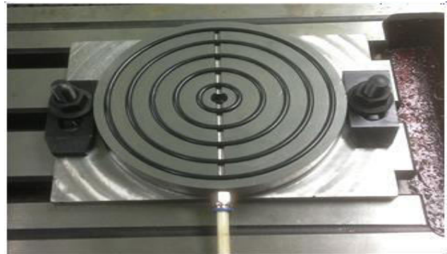
Figure-2.3. The vacuum clamping on a milling machine.
