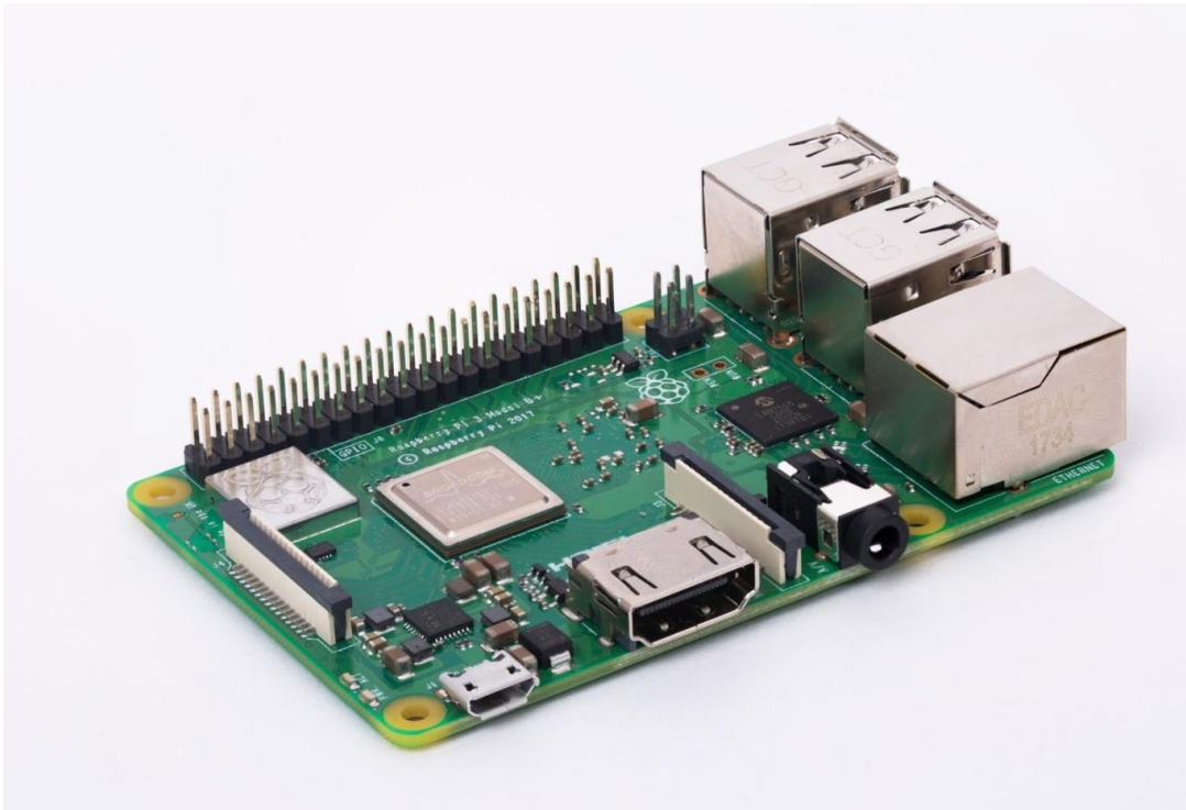
Figura 22: Raspberry Pi 3 Model B+.
