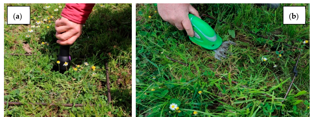
Figure 2. Portable near-infrared (NIR) sensor measurement (a) and pasture sample cut (b).
