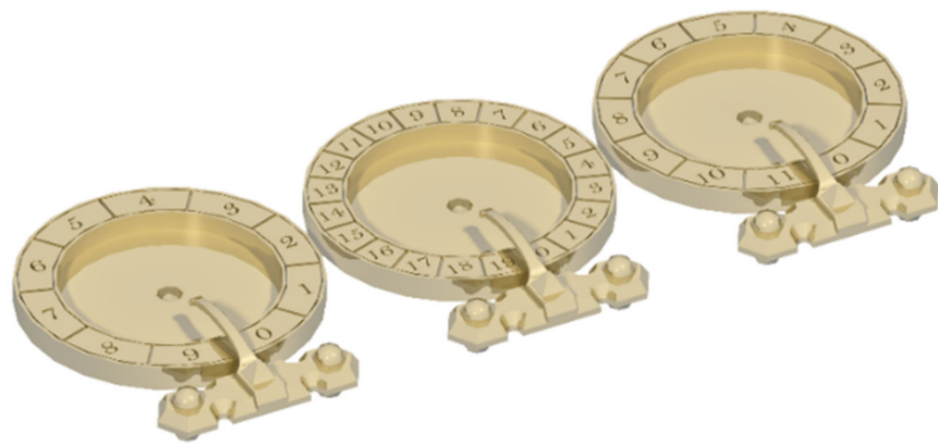
Figure 19. Models of the numbered crowns together with the stop bars in their real relative position.
