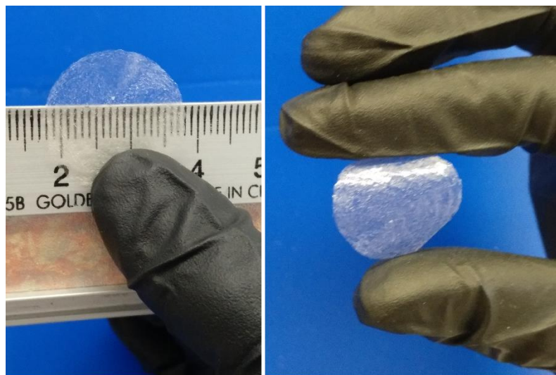
Figure 6. 3D printed CHI2PEC2 scaffold after drying at room temperature.
