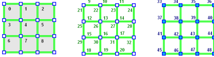
Figure 1: Coding of the cubes in a 3 \times 3 picture (2-cubes on the left, edges on the center and vertices on the right).
