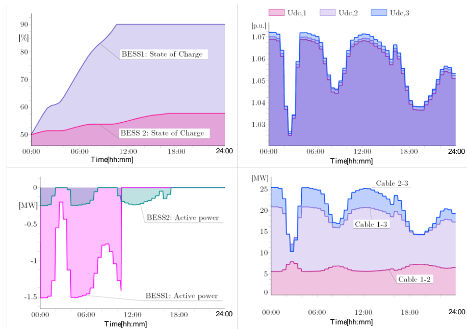
Figure 14. Simulation results: BESS1 and BESS2, P_{dc,set1} = -5 MW, P_{dc,set2} = +5 MW, and \rho_{dc1} = \rho_{dc2} = 0.005 pu/MW. Low wind speed.
