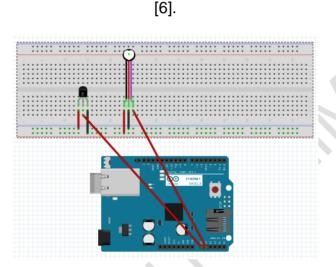
In Figure 16 you can see the circuit with the temperature and heart rate sensor, together with an arduino uno with its respective Ethernet shield to connect to a router and send the data obtained to the Ubidots platform.
