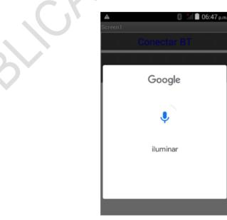
In Figure 8 you can see the execution of the illuminate command on the mobile phone using the program made in the MIT App inventor.
