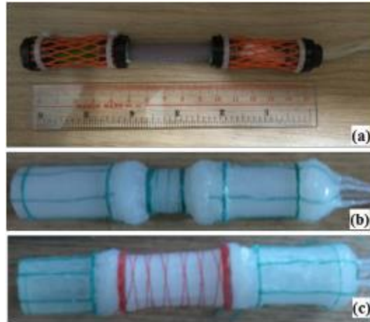
Figure 2-4: Prototypes of the soft earthworm robot: (a) Version 1; (b) Version 2; (c) Version 3 (Heung, Chiu, and Li 2016)
