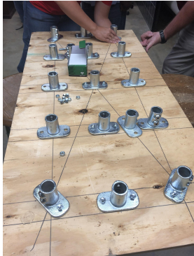
Figure 8. Arrangement of mounted galvanized floor flanges for the various array configurations
