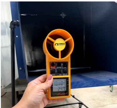
Figure 9. The wind tunnel at Georgia Southern University, with the anemometer reading 10.4 m/s.
