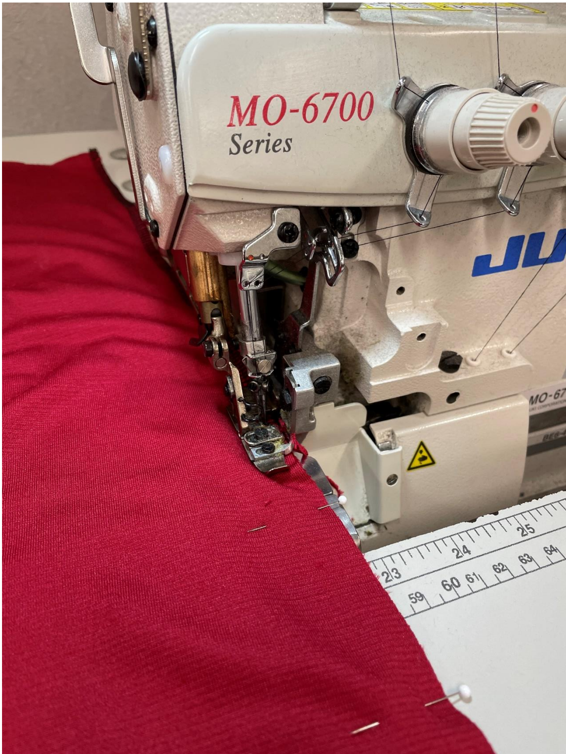
Figure 25 When sewing knit fabrics, I used the serging machine instead of a regular straight stitch sewing machine to ensure that the seams do not pop, they stretch with the fabric.
