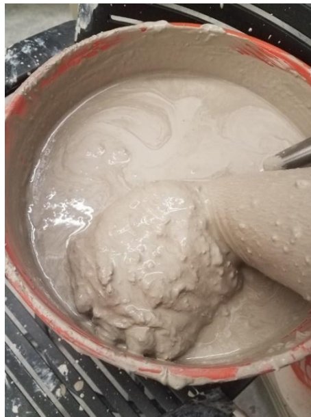
Figure 14. Slip materials mixed with a small amount of water- not sieved.
