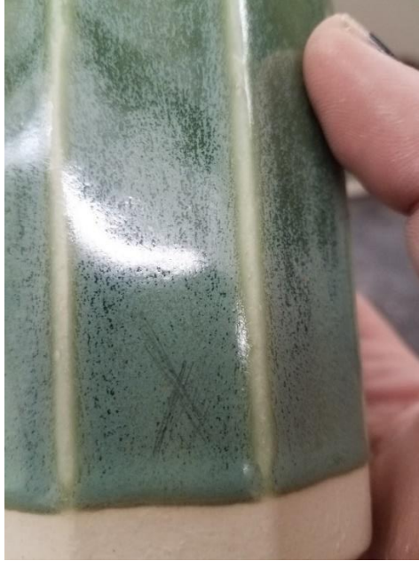
Figure 42. An “X” on a soft glaze showing the results of a cutlery marking test.
