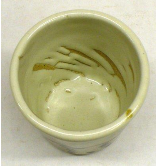
Figure 3. Example of crawling (Photograph by Tony Hansen. “Crawling” Digital Fire , 2018.) 20
