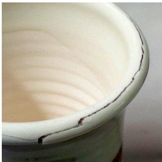
Figure 6. Example of shivering (Photograph by Tony Hansen. “Shivering” Digital Fire , 2018.) 27
