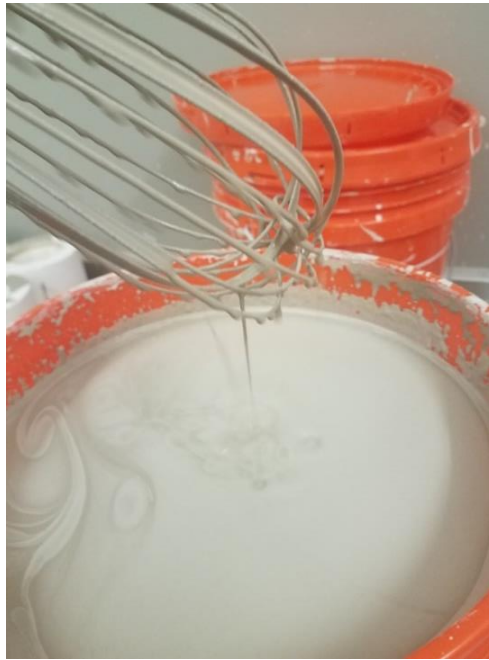
Figure 15. Slip at a cream consistency-streaming smoothly off the whisk without clumps.
