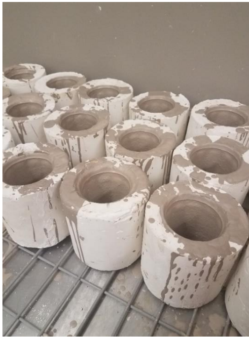
Figure 17. Emptied plaster molds with a layer of slip drying along the inside form.
