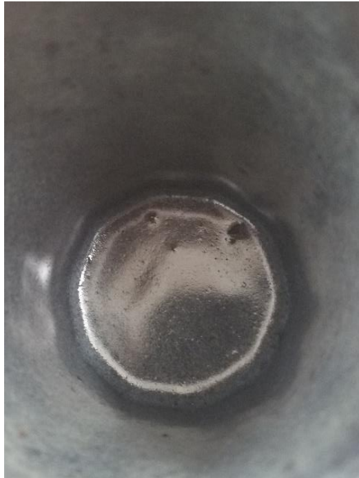
Figure 37. Pinholing and small blistering of the re-tested Licorice glaze.
