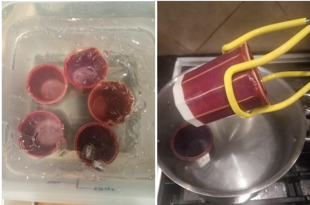
Figures 44-45. The process of the boiling water: ice water test.
