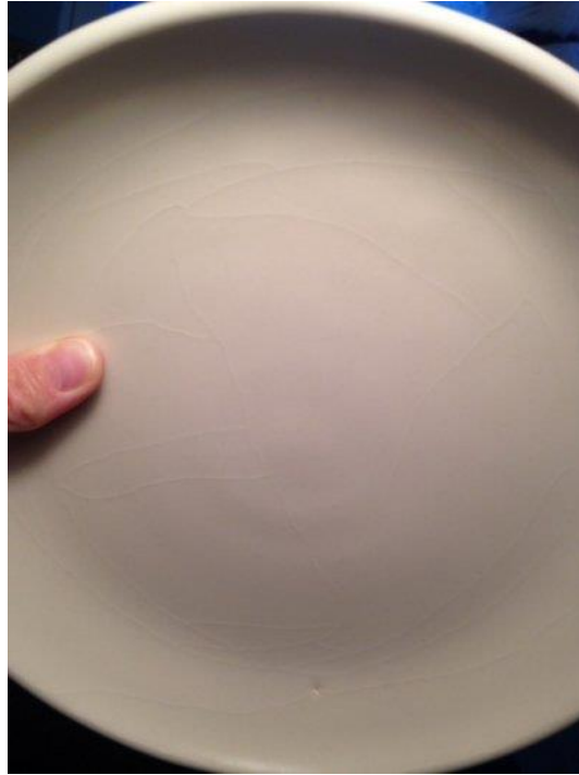
Figure 5. Example of crazing (Photograph by Tony Hansen. “Crazing” Digital Fire , 2018.) 25
