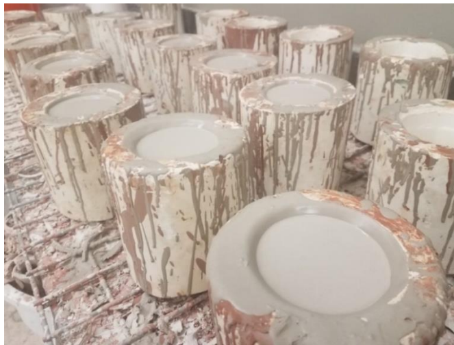
Figure 16. Plaster molds filled with slip.
