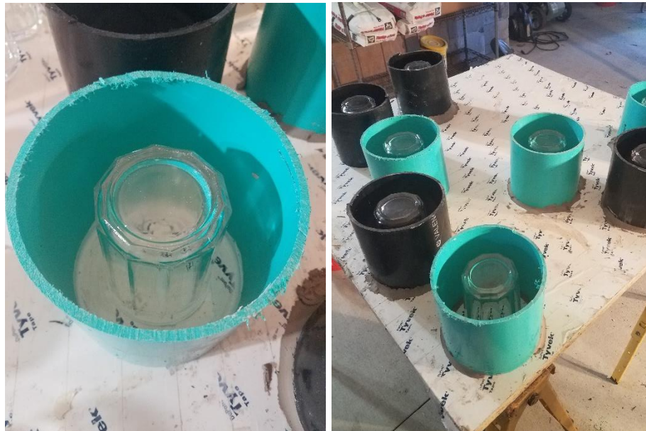
Figures 11-12. The glass cups and garden irrigation pipes secured to the table with clay and silicone.
