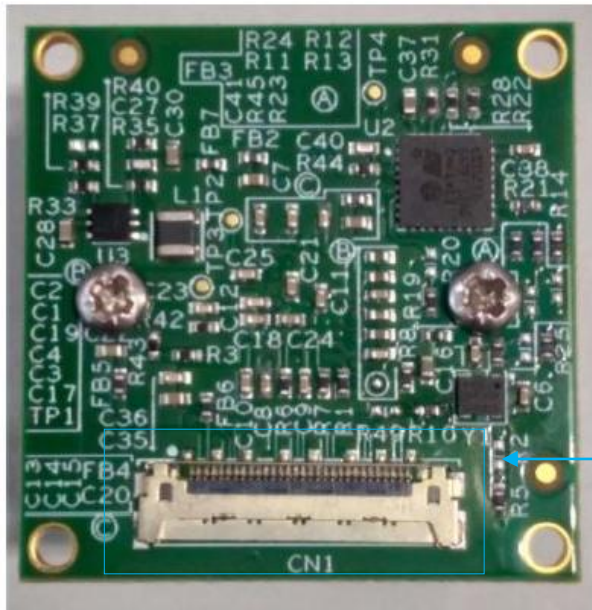
Figure 2: Rear View of e-CAM222_CUMI2311_MOD Camera Module
