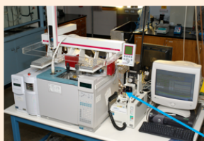
TD-Py-GC-MS consists of CDS Analytical 5200 Pyrolyzer connected by transfer line to GC inlet
