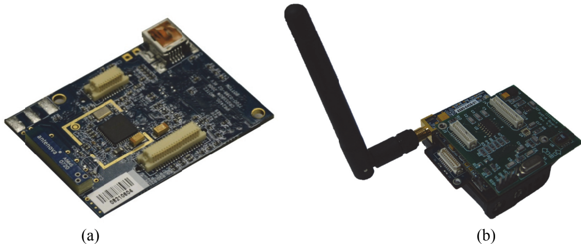
Figure 1: (a) Imote2 (b) Imote2 and ISM400
