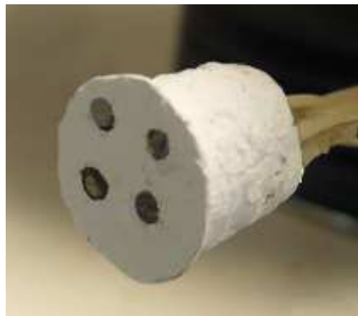
Figure 4. In house constructed resistivity probe
