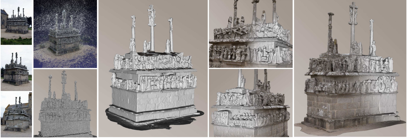
Figure 2. From left to right: three of the 27 images (8 Mpixels) of a sculpted calvary taken from the ground; the generated point cloud (1,300,000 points) and visibility consistent mesh M^0 (1,200,000 triangles); final reconstruction (1,850,000 triangles); close views of the final reconstruction with and without texture remapping. Note the high percentage of outliers in the point cloud and to what extent M^0 is noisy but close to the solution in position and topology.
