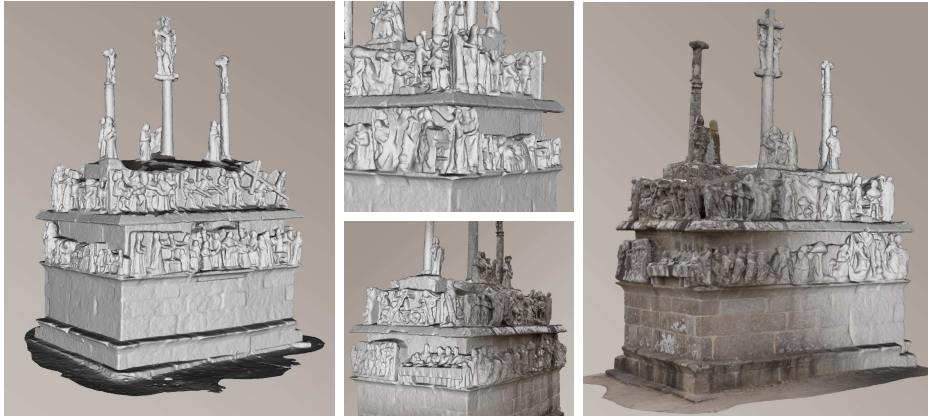
Figure 4.5: calvary data set . From left to right: two of the 27 images (8 Mpix) of a sculpted calvary taken from the ground, the generated point cloud (1,300,000 points), the initial mesh \mathcal{S}^0 (1,200,000 triangles) and the final reconstruction (1,850,000 triangles).
