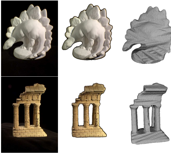
Figure 4.1: Visual hull. Objects acquired under controlled imaging conditions from Seitz et al. [2006] , silhouetted images and the corresponding (approximated) visual hulls. While the visual hull does not capture deep concavities (the temple’s stairways or the dino’s legs, for instance), it already provides a good initialization for variational methods.
