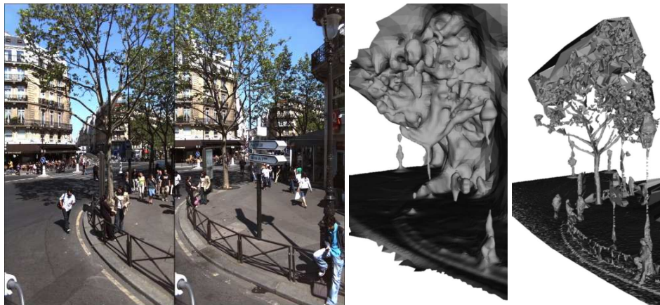
Figure 3.17: Reconstruction details of the rue Soufflot: acquired images (left), corresponding reconstruction results of Poisson (center) and our method (right).
