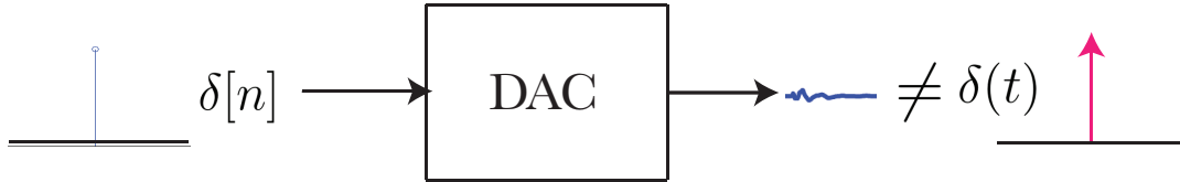
Figure 3.3: Kronecker Delta after Digital-to-Analog Conversion
