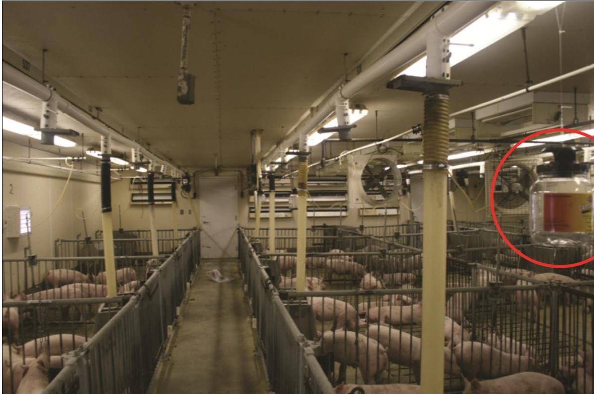
Figure 6. Setup of volatile preference experiment. Starbar® CAPTIVATOR® fly traps were attached to pipes on the ceiling and filled with Pinot Noir red wine, a swine feed and water mixture, apple cider vinegar, or left empty as a control.
