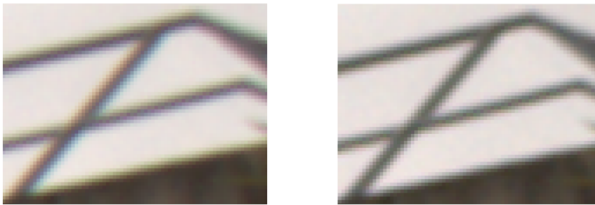
Fig. 1. Cropped and zoomed-in image from camera Canon EOS 40D, before (left) and after (right) chromatic aberration correction by our method. Notice the attenuated color fringes at edges between left and right images.
