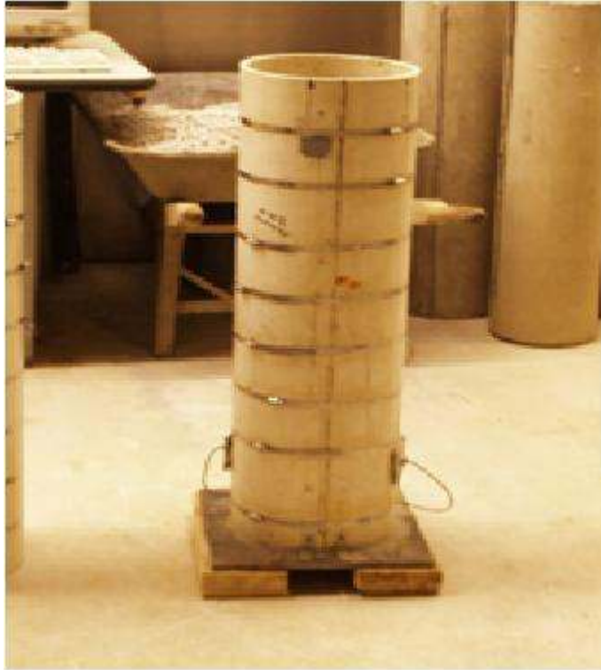
Figure 3.5. Formwork pressure test column [21].
