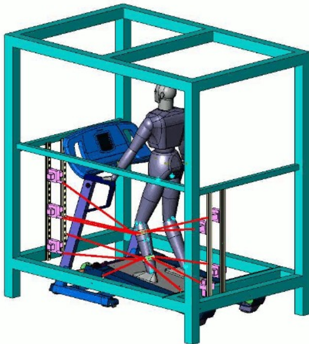
Figure 3.3: A CAD model of the MARIONET-REHAB frame, with the passive wire sensors shown
