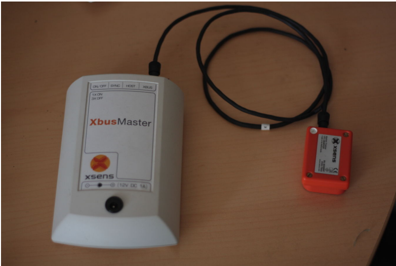
Figure 3.5: The Xbus Master along with a MTx inertial measurement unit, which is the main unit mounted on the collar
