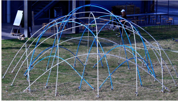
Figure 22: View of the interweaving grid on the ground and of the two interconnected gridshells
