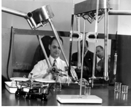
Figure 1.3: Raymond Goertz operating a mechanical teleoperator. He later invented the first electro-mechanical master/slave teleoperator. (Source: Argonne National Laboratory).
